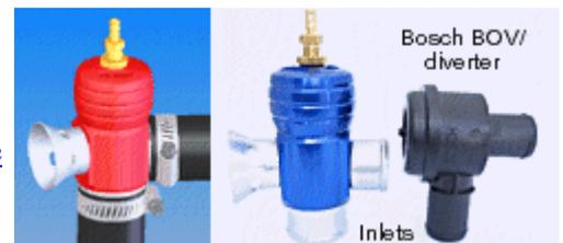
Be careful about the orientation of the valve when the factory inlet and outlet hose are the same diameter. The majority of European manufacturers install their diverter valves in the opposite orientation to the way a GFB valve should be installed. Boost should always enter the bottom of a GFB valve, and dump through the side outlet(s).
