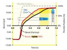
("Chart shows comparative manifold boost pressure rise during 1st to 2nd gear shift as tested on a CA18DET with a 128 turbo GFB TMS improvement is seen as a 30% faster return to peak boost, during which time up to 40% more boost is available)
