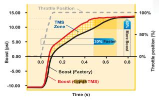
(\*Chart shows comparative manifold boost pressure rise during 1st to 2nd gear shift as tested on a CA18DET with a T28 turbo. GFB TMS improvement is seen as a 30% faster return to peak boost, during which time up to 40% more boost is available)
